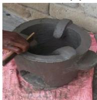
Next, we need to add the 3 supporting legs on which the stove will sit. We can also add the 2 handles at this stage. There is a special measuring disk which shows the correct way to attach these appendages. Simply mark on the clay where each attachment will go.
